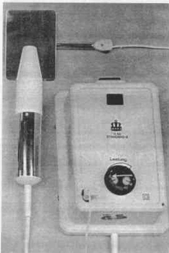
Figure 1. High Frequency Oxygen Therapy apparatus: TEFRA N53 Standard III with hand and flat electrodes.
